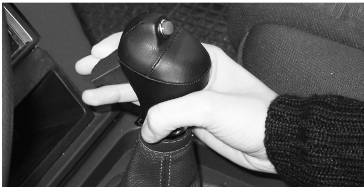
Total Ability: Electronic Clutch
