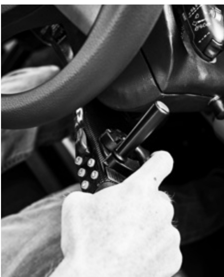
Total Ability: Brake Levers
