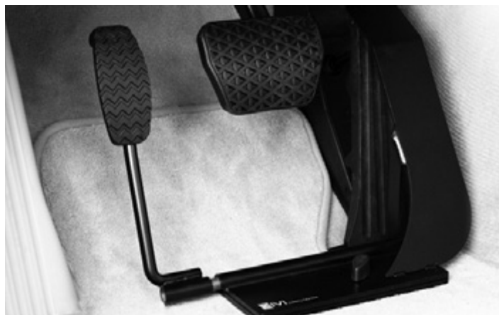
Mobility Engineering: Left Foot Accelerator
