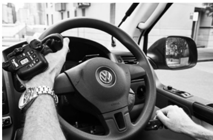
Total Ability: Satellite Accelerator
